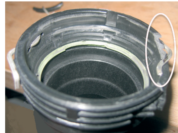
Component failure in the area of a clamping bracket
